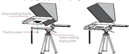
• Likewise, fix the self-inspection display to the plate by using thumb screws.
