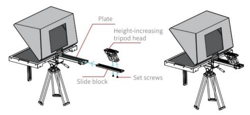
• Fix the quick mounting plate at the bottom of the camcorder, and install the camcorder to the top of the height-increasing tripod head.
