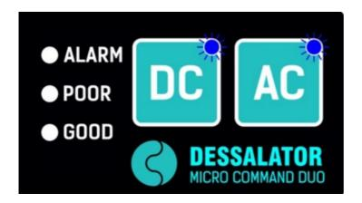
To STOP your watermaker normally: If you run on DC power press and hold the button for about 2 seconds. If you run on AC power press and hold the button for about 2 seconds. Upon release of the button, the watermaker will STOP and go to STANDBY.
