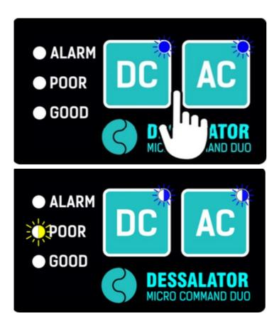
To start the watermaker from STANDBY and run it on DC power, press and hold for about 2 seconds. To start the
