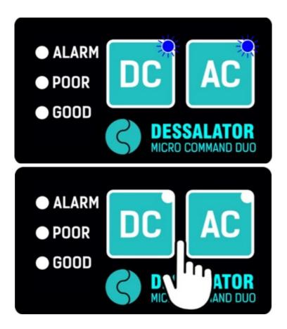
When your watermaker is in STANDBY, both BLUE LEDs are lit as an indication. Should these BLUE LEDs be perceived as disturbing, they can be turned off by briefly pressing one of the buttons. Another brief press on one of the buttons will turn the BLUE LEDs back on if the watermaker is still on standby
