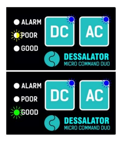
The RED, YELLOW and GREEN LEDs will show the same indication as on the control panel of the watermaker. The blinking speed of the YELLOW LED provides feedback of the water pressure in the system: faster blinking means higher pressure. The BLUE LED that is lit shows if the machine is running on DC or AC power. Once the production water is of good quality, the GREEN LED will light up.
