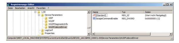
To set the DWORD registry value, the device needs to be connected, so that the driver can be included in the Windows registry. As soon as the value is set, the device must be logged on to the USB interface once again. This can either be done by connecting/disconnecting the USB cable or by disabling and re-activating the driver.
