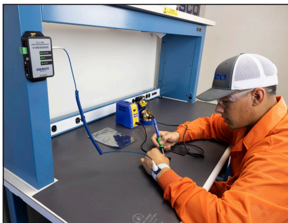
Figure 10. Using the Full-Time Continuous Monitor when mounted on a workbench upright
