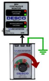
3. Set the rotary switch to OPERATOR FAIL LOW.
