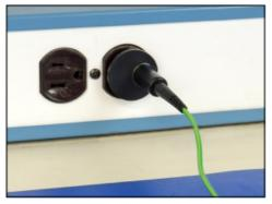
2. Insert the verification tester's black operator test lead into the Mini Monitor's operator jack.
