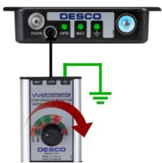
3. Set the rotary switch to OPERATOR FAIL LOW.
