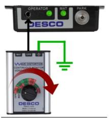
3. Set the rotary switch to OPERATOR FAIL LOW.
