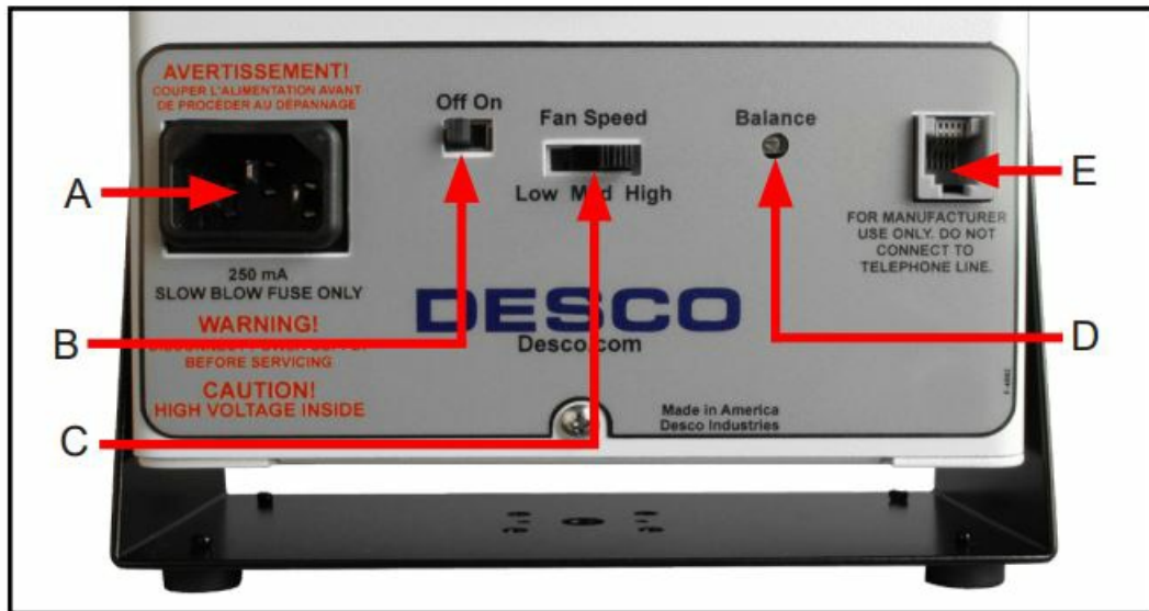
Figure 2. High Output Benchtop Ionizer features and components
