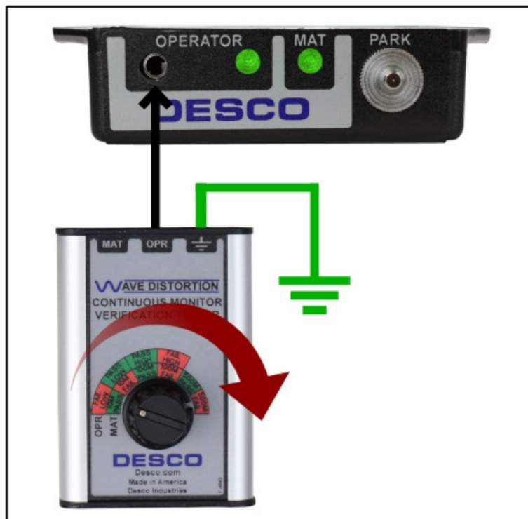
Figure 6. Connecting the Wave Distortion Monitor Verification Tester to the Multi-Mount Monitor's operator jack
