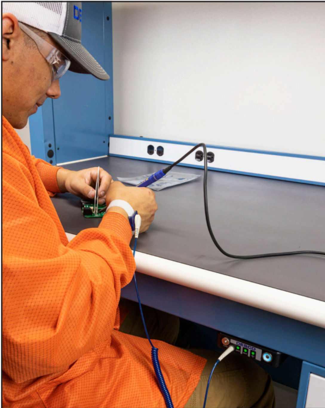
Figure 9. Using the Full-Time Continuous Monitor when mounted underneath a workbench tabletop
