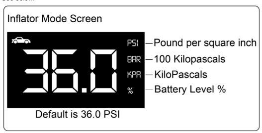
5. The default setting is 36.0 PSI. To change from PSI/BAR/KPA simply press the "Inflator mode" with a single press.
