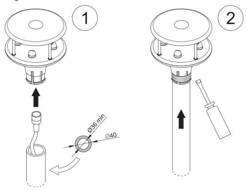
The support mast, having a 40 mm maximum outer diameter and 36 mm minimum inner diameter, should be positioned on a stable surface.
