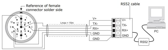
To use the RS52 cable, the drivers included in the HD52.3D-S software package should be installed in the PC (see the guide to USB drivers installation included in the software package). The instrument is powered directly from the USB port of the PC.
