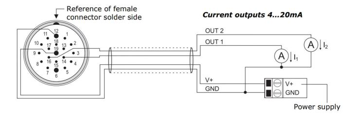
Current outputs are active. Load resistance: RL < 300  $\Omega$ .
