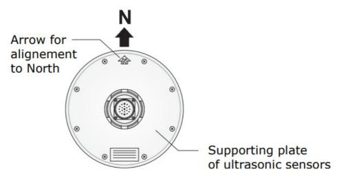
For an accurate alignment, connect the instrument to a PC (see following chapters for communication protocols), then rotate the instrument on its vertical axis until the compass measures  $0.0^{\circ} \pm 0.1^{\circ}$ .
