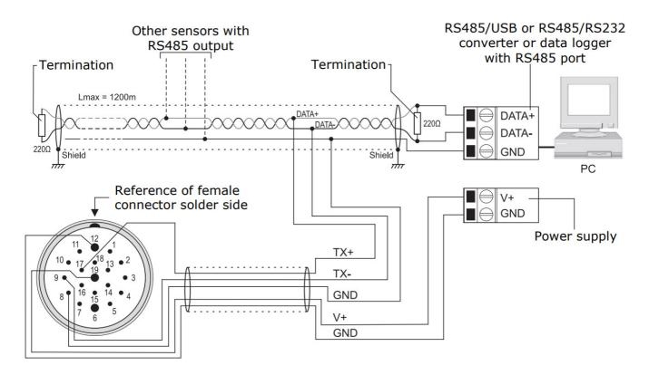
Thanks to the RS485 connection, multiple instruments can be connected to a multi-point network.
