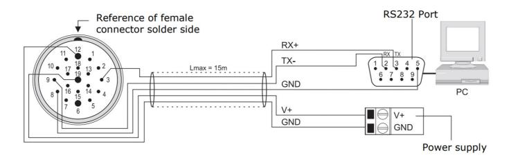
For RS232 connection, TX-, RX+, and serial GND signals (pin 9, 3, and 8 of M23 connector) are used, to be
