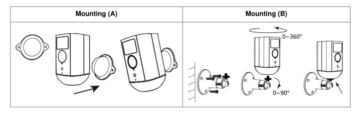
B. Adjust the camera angle by aiming and rotating it. Fasten the screw.
