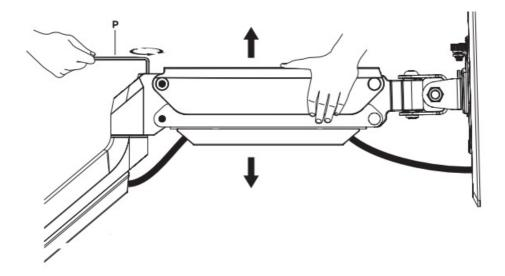
Hold the monitor arm horizontally to avoid damage to monitors or monitor arm. Ask for help from a 2nd person if needed.
