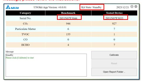
2. For the first-time use or when replacing the standard machine, please set the [Benchmark Calibration Date] according to the benchmark information.
