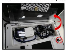
2. Ensure all dip switches on the Benchmark are down, then install it on the left and the test device (DUT) on the right. Connect the UNOnext with the 14-pin cable and the UNOlite with the 5-pin cable. Close the chamber to complete the installation.
