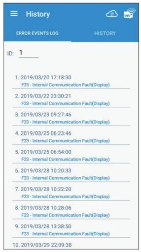
Details can be verified in the "ERROR EVENTS LOG" pages. Refer to the Manual of the Inverter for details on the error codes.
