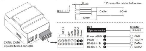
2. Hold down both side ① of the 16-pin connector, insert cables and then connect to Data Collector.
