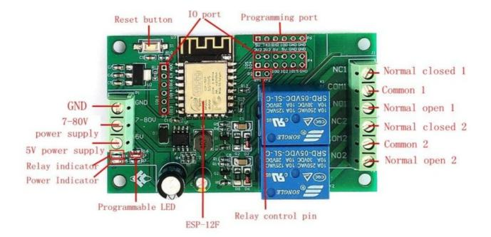
Programming port: ESP8266's GND, RX, TX, 5V are respectively connected to the GND, TX, RX, 5V of the external TTL serial port module. IO0 needs to be connected to GND when downloading, and then disconnect the connection between IO0 and GND after the download is complete;
