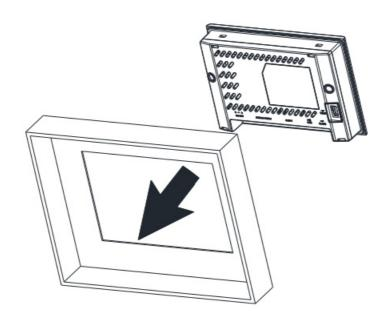
**Step 2:** Place the fasteners into slots and tighten the screws till reaching the panel cutouts.
