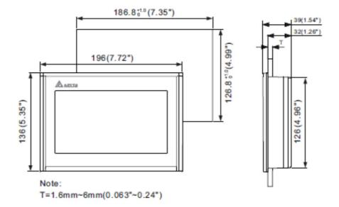
Operation Temperature is  $-30^{\circ}$ C  $\sim +70^{\circ}$ C Storage Temperature is  $-40^{\circ}$ C  $\sim +80^{\circ}$ C
