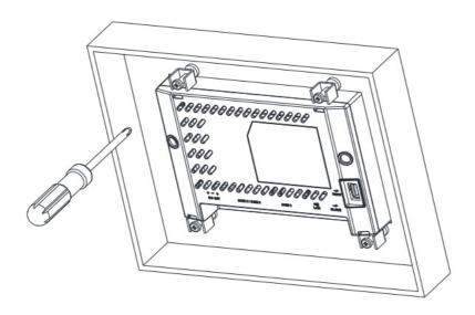
**Step 4:**For heat dissipation, keep a minimum clearance of 60 mm (2.36 inches) and 45 mm (1.77 inches) respectively on the rear and bottom of the HMI.
