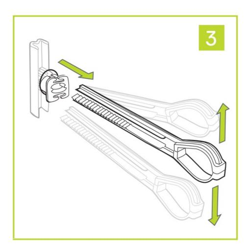
4. Place thumb between straps at wall. Push thumb side to side, snapping off straps level with flange of cap.
