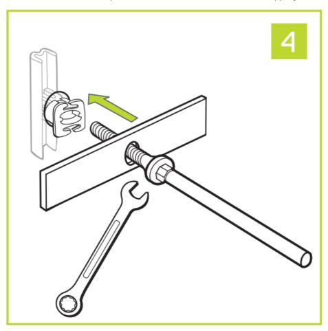
5. Insert Invisibolt bolt through white flat washer and tighten until snug, then stop. Use wrench to tighten securely. Be careful when finding the thread, inserting the Invisibolt with too much force can push the channel through
