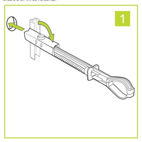
2. Drill 5/8" (15mm) hole. Hold metal channel alongside plastic straps & slide channel through the hole. Minimum clearance behind wall: only 1-7/8".
