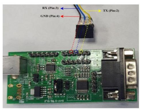
The above image shows the connection of UART to the USB conversion board for accessing console logs. The Tx, Rx and GND pin needs to be connected to the respected marked circles in the H7 connector of the U2UC board.
