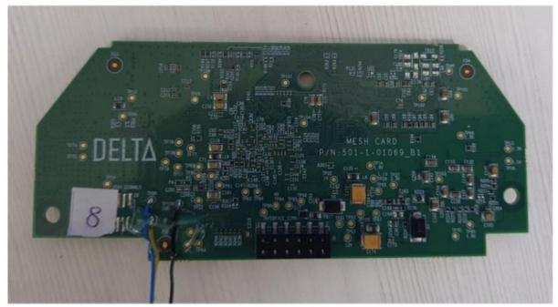
The Bottom Side of the Mesh Card contains the IO connector (PCB Ref Des J5) used to provide a supply to the board and communicate with the meter over UART serial interface.
