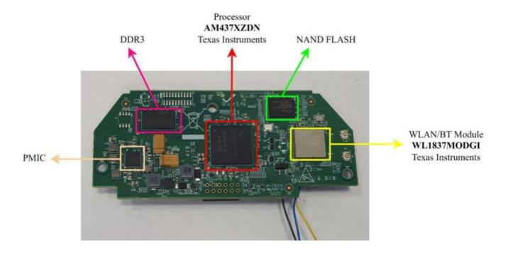
• The top side of the Mesh Card contains the Main Processor AM437XZDN, Wi-Fi Module WLAN/BT Module WL1837MODGI, DDR3, and PMIC.
