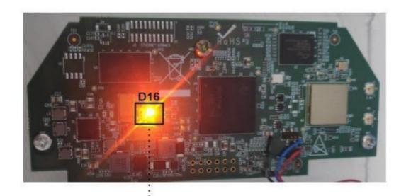
When board is powered ON D16 LED (in top of mesh card)will glow
