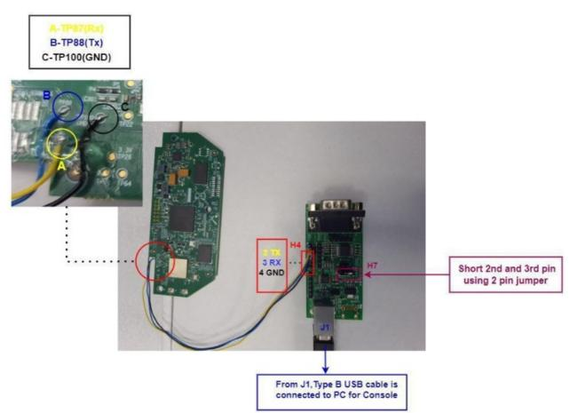
Step 1: The UART signals are taken from the Test points of the Mesh card as follow,
