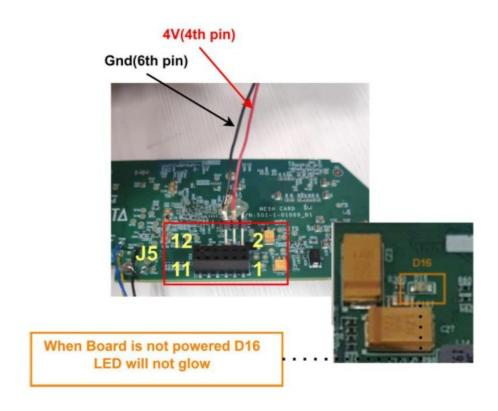
**Step 1:** Connect the male header to the respective female header(J5) in the board.
