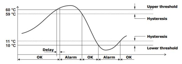
Enabling the Buzzer Latch option, the buzzer continues to sound even after the alarm condition has ceased. In the event of an alarm in progress with the buzzer active, the buzzer can be silenced for a configurable time. Once the set time has elapsed, the buzzer will resume sounding or not depending on whether the alarm condition is still present or not.
