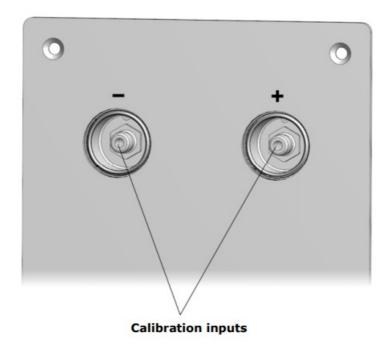
The differential pressure zero calibration is also possible via the Modbus Coil register with address 72 (see chapter 8).
