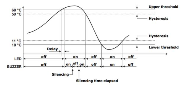
The following example shows the silencing of the buzzer with Latch option enabled.
