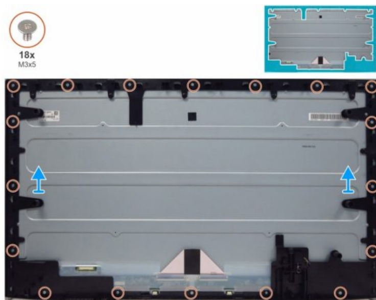
Figure 7. Removing the middle frame
