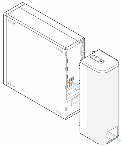
4. Align the cable cover retaining hooks with the slots on the chassis.
