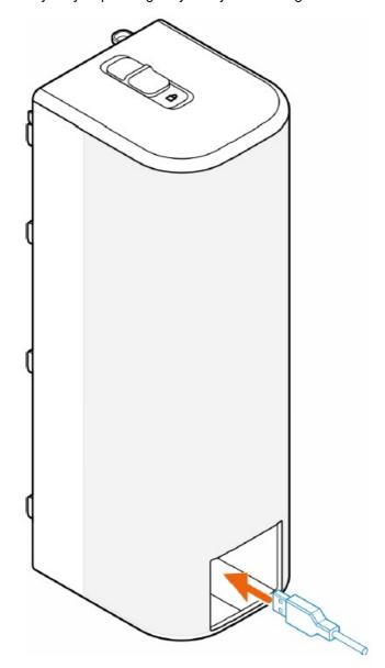
$\ensuremath{\mathsf{3}}.$  Connect the cables to their respective ports on the chassis.
