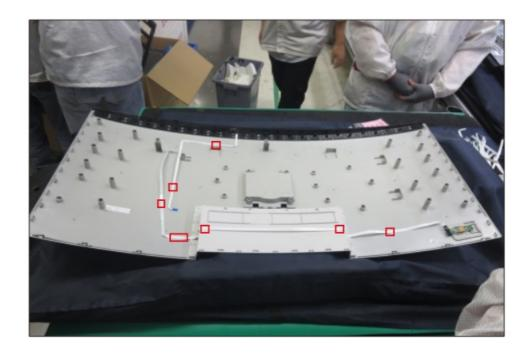
Move the assembled rear cover close to the panel unit, then connect the joystick key cable and sensor cable to the connectors of interface board. Put down the rear cover and push the rear cover on the positions marked as the picture below shown for mechanisms engagement.
