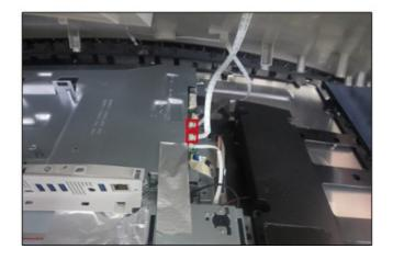
Release the cables by tearing off all the tapes. Use a Philips-head screwdriver to remove 2pcs screw for unlocking the joystick board, then release the joystick board sensor board from the hooks of the rear cover.(No.1~2 screw size=M2x2.4, Torque=1±0.2kgfxcm)
