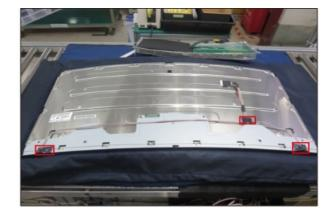
Take 1pcs LED board and 1pcs middle frame, and then locate the LED board into the specific position of the middle frame. Paste 1pcs mylar tape to fix the LED board, then fix the LED cable on the middle frame by the double-faced tape on the back of the cable.
