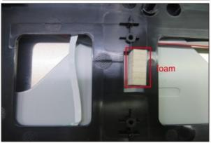
Move the bracket chassis module close to the panel module, then connect the eDP cable to the connector of the panel, then put the bracket on the back of the panel module.
