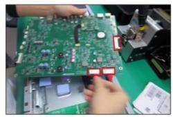
Turn over the interface board and locate it into the bracket, then use a Philips-head screwdriver to tighten 4pcs screws for locking the interface board.(No.9~12 screw size=M3x6, Torque=5±1kgfxcm)
