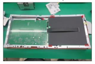
Panel preparation: Take out 1pcs panel module from the carton, remove the protective film by tearing off all the tapes of screen, then examine the panel surface according to inspection criteria carefully.
