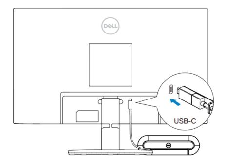
**NOTE:** If the speakerphone is not detected, check if the upstream cable is connected from your computer to the Dell monitor.
