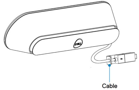
2. Dislodge the USB-A connector from the adapter as required
