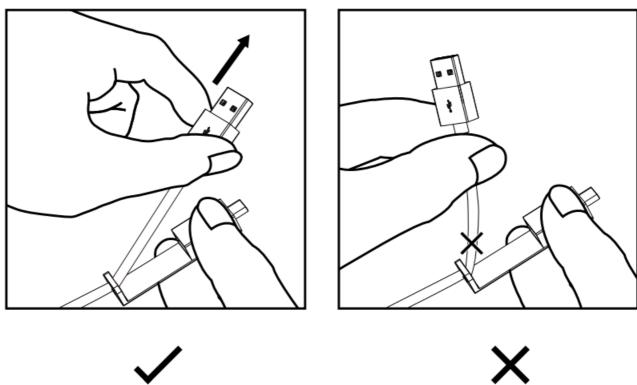
Caution: Bending the cable at a sharp angle could damage the cable and cause it to fray overtime.
