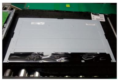
S15 Remove the black Mylar sheet from the hooks of the main bracket as the picture below shown.
