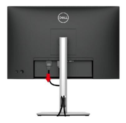
S3 Remove stand from the product.(Press the stand release button, lift the stand up and away from the monitor)
