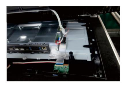
S7 Put the rear cover into a fixture jip, then release the key cable by tearing off the tapes. Use a Philipshead screwdriver to remove 1pcs screws for unlocking the joystick key board with the rear cover. (No.1 screw size=M2x3.3,Torque=1±0.2kgfxcm)
