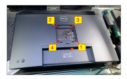
S5 Wedge your fingers between the rear cover and the middle bezel on the corners of the top side of the monitor to release the rear cover, then use one hand to press the middle bezel, the other hand to pull up carefully the rear cover in order of arrow preference for unlocking mechanisms of rear cover..
