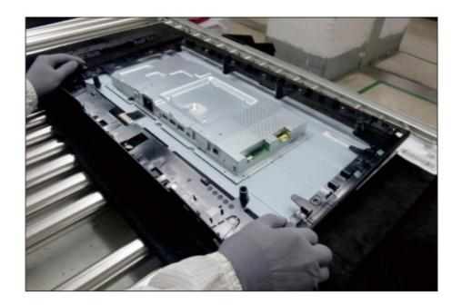
S13 Use a Philips-head screwdriver to remove 2pcs screws for unlocking the bracket chassis with the panel. (No.1~2 Screw size= M3x3, Torque=5±1kgfxcm)
