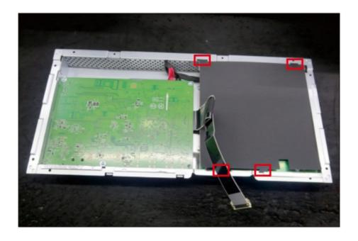
**S16** Use a Philips-head screwdriver to remove 5pcs screws for unlocking the power board and interface board, and then release all the cables from the hooks.
