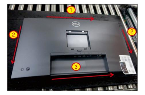
S6 Lift the rear cover up carefully. Disconnect the joystick cable from the connector of the interface board, and then remove the rear cover.
