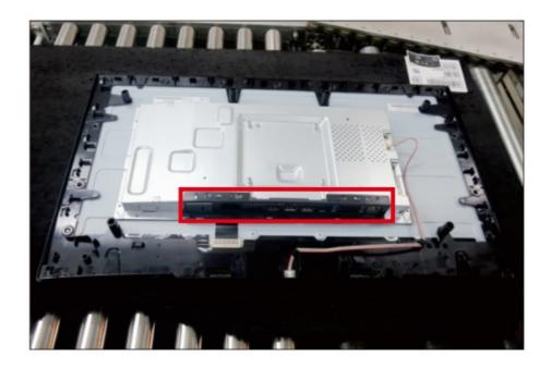
S11 Disconnect the panel lamp cable from the connectors of the panel and interface board, then tear off the tapes and release the lamp cable from the hook of middle frame.
