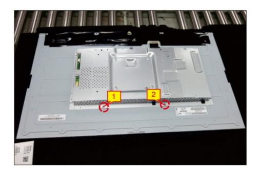
S14 Push the earing -locks and disconnect the LVDS cable from the connector of the panel module, then lift up and take away the bracket chassis module and then put it on a cushion for later disassembling.
