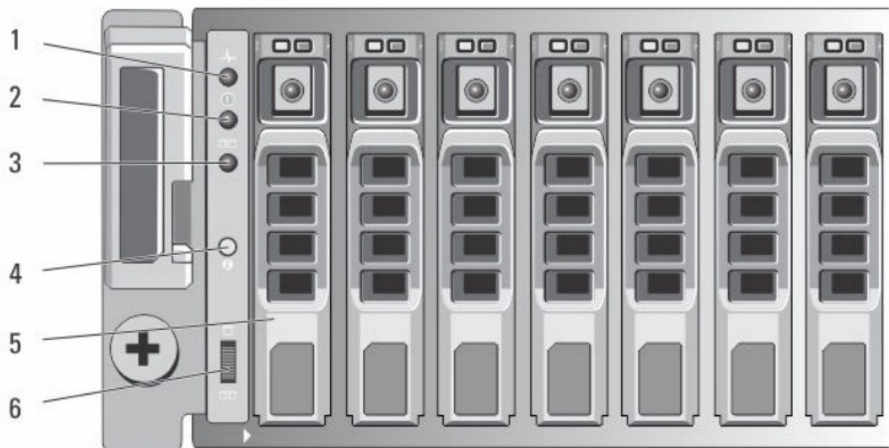
Figure 2. Front-Panel Features and Indicators—Dell PowerVault MD3820i
