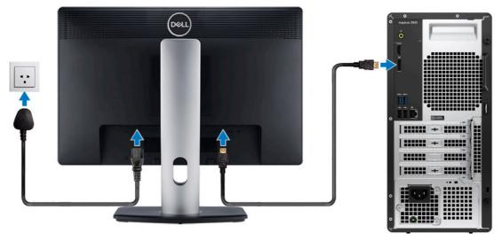
NOTE: The location to connect the display cable can vary if your computer has a discrete graphics card installed. For optimal graphics performance, ensure to connect the display cable to the graphics card if there is one installed.
