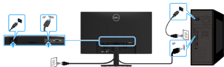
Figure 7. Connecting DP cable
