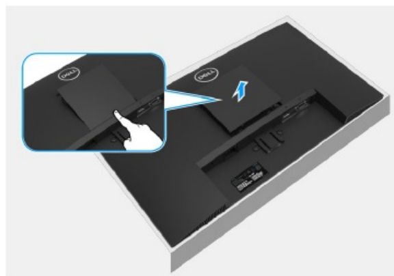
Figure 10. Removing the VESA cover
