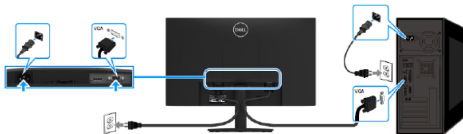
Figure 6. Connecting VGA cable
