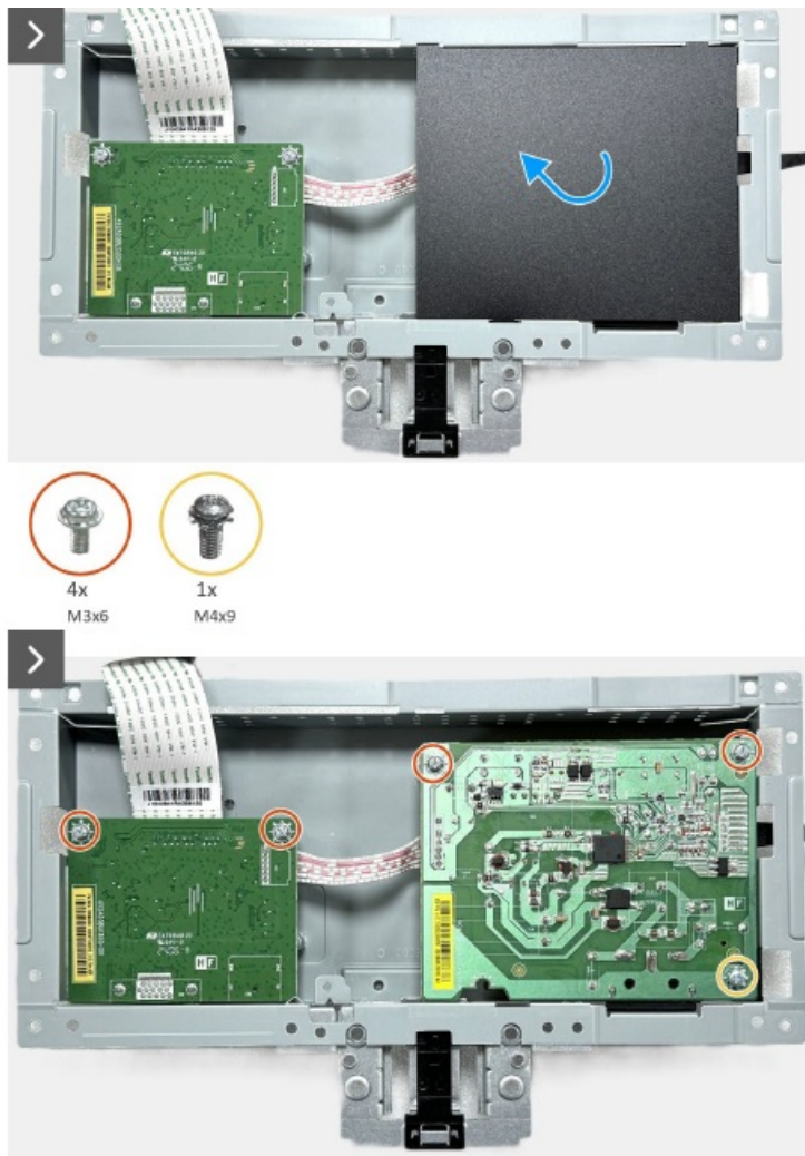
Figure 20. Removing the interface board
