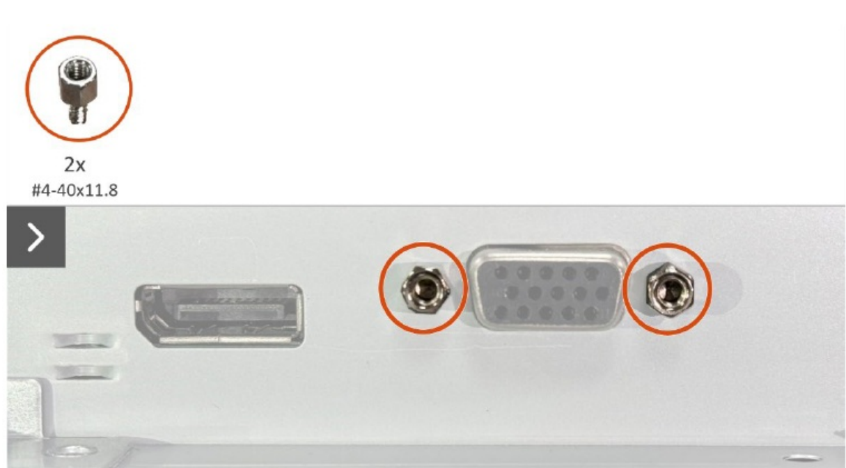
Figure 19. Removing the interface board
