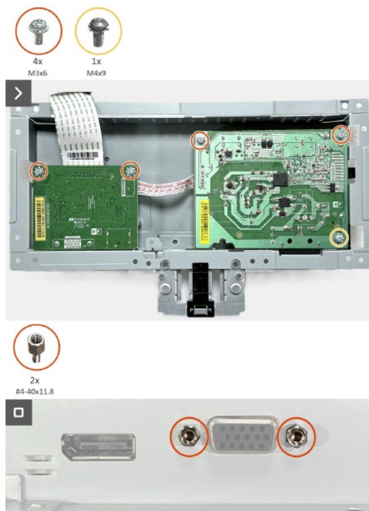
Figure 23. Installing the interface board
