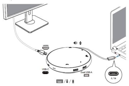
3. MH3021P supports power delivery up to 90W when connected to the Thunderbolt or USB-C (Display Port Alt Mode) port of your PC. Power source can be supplied by the USB-C power adapter or USB-C monitor that support charging feature. Below two images show MH3021P connected to an external power source via USB-C power adapter or USB-C monitor.
