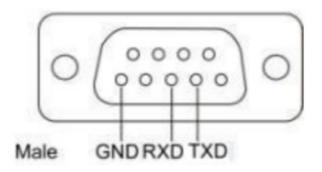
This display uses RXD, TXD, and GND lines for RS-232 control.
