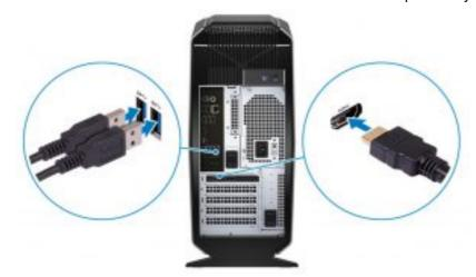
**NOTE:** Connect the headset to the HDMI port on the primary graphics card and connect the display to any available port on the card.
