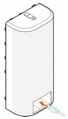
3. Connect the cables to their respective ports on the chassis.
