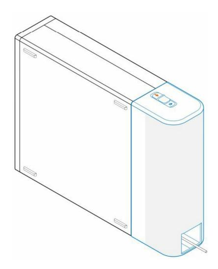
**NOTE:** For added security, use the Kensington cable lock to secure the computer.
