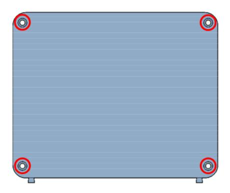
Find the place where you want the control unit installed. The control unit is mounted using four screws, one in each corner.
