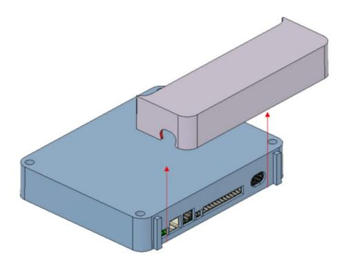
Remove the connector cover by sliding it off vertically.
