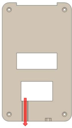
If installation is done without having the cable coming in from behind the display, place the cable inside the groove of the backplate as shown in the picture above.
