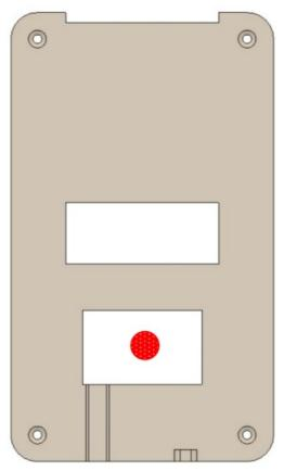
Make a hole for the cable in the lower square on the back plate like shown in the picture above. We strongly suggest that you use a cable without connectors to prevent damage to the connectors when pulling it through the wall.
