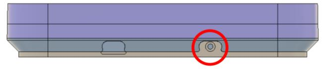
Slide the back plate down so that it comes free from the hooks in the display case and then remove it
