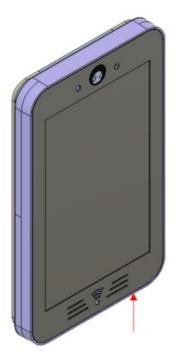
Put the security screw back (from Step 1) to secure the display after mounting.
