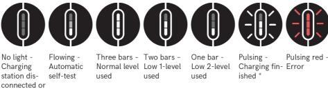
Pulsing with one, two or three bars depending on chosen level.
