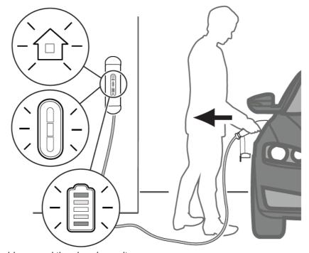
2. Coil the charging cable around the charging unit.
