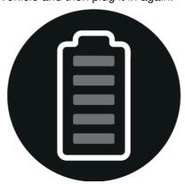
This error state will display if there is a problem on the vehicle side. This could be caused by the cable not being connected correctly, a faulty or damaged vehicle connection or a damaged cable plug.
