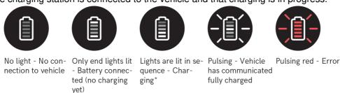
• The speed in which the lights are lit indicates which charging level is used.
