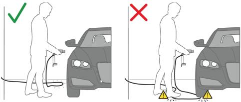
Always hold the cable by the handle when pulling it. Do not pull the cable itself.
