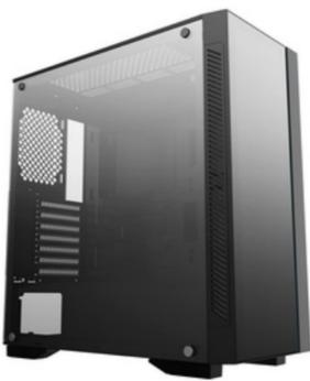
DeepCool Matrexx 55 V3. Form factor: Midi Tower, Type: PC, Product colour: Black. Power supply location: Bottom, Supported power supply form factors: ATX, PS2. Front fans diameters supported: 120,140 mm, Rear fans diameters supported: 120 mm, Top fans diameters supported: 120,140 mm. Supported HDD sizes: 2.5,3.5". Width: 210 mm, Depth: 446 mm, Height: 479 mm **Design**
