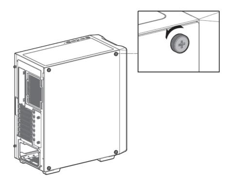
**Removing the Metal Side Panel**
