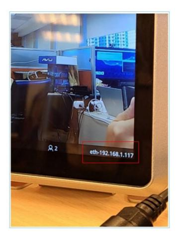
After powering ON the AITP04 unit, wait till the assigned I.P address from the DHCP server shows on the bottom-right side of the AITP04 display screen.
