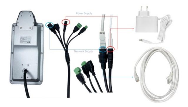
Plugin the RJ-45 Ethernet and power supply cables into the AITP04 unit and power ON the AITP04 unit **Note:** The other end of the power supply cable must be connected to the power supply. The other end of the RJ-45 should be connected to a LAN-connected router, bridge or switch.
