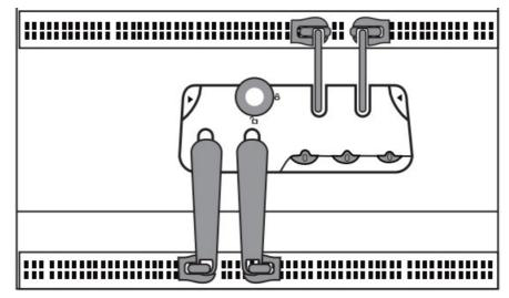
**Step 2:** Press down the reset button with a tool until a "click" sound
