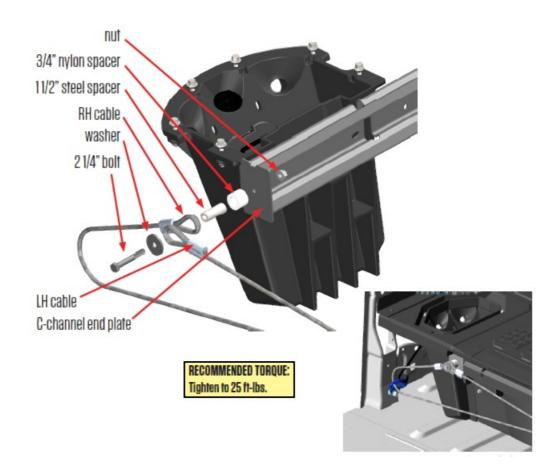
Enlargement of RH cable assembly attachment to cargo tie down loop.
