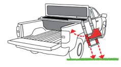
PLACE LADDER ON SOLID GROUND WITH BOTH RUNGS LOCKED INTO PLACE (LADDER STEPS 1-3). FAILURE TO DO THIS COULD ALLOW LADDER TO SWING INTO TRUCK AND CAUSE DAMAGE TO THE VEHICLE
