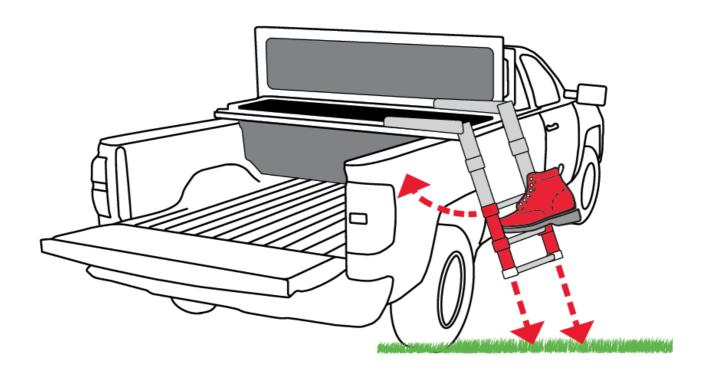
PLACE LADDER ON SOLID GROUND WITH BOTH RUNGS LOCKED INTO PLACE (LADDER STEPS 1-3). FAILURE TO DO THIS COULD ALLOW LADDER TO SWING INTO TRUCK AND CAUSE DAMAGE TO THE VEHICLE
