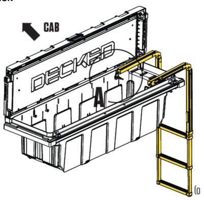
1. Check to see that the ladder pivot brackets are installed – (orange in Detail A). If not, see the previous page.
