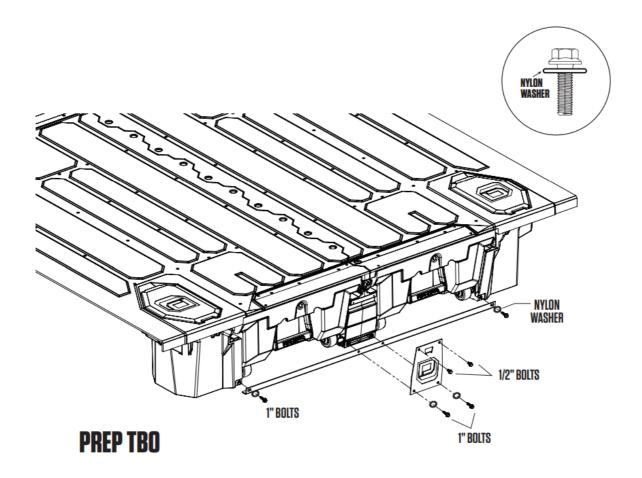
**HELPFUL TIP:** The bottle opener goes on the outside of the torsion brace. **RECOMMENDED TORQUE:** 1" Bolts – 27 in-lb. | 1/2" Bolts – 18 in-lb.
