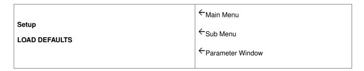
When highlighted in the Main Menu, press the ENTER button to enter this sub-menu. Press the < and > buttons to move left or right respectively through the 6 menus below and press the BACK button to go back to the Main Menu when finished.
