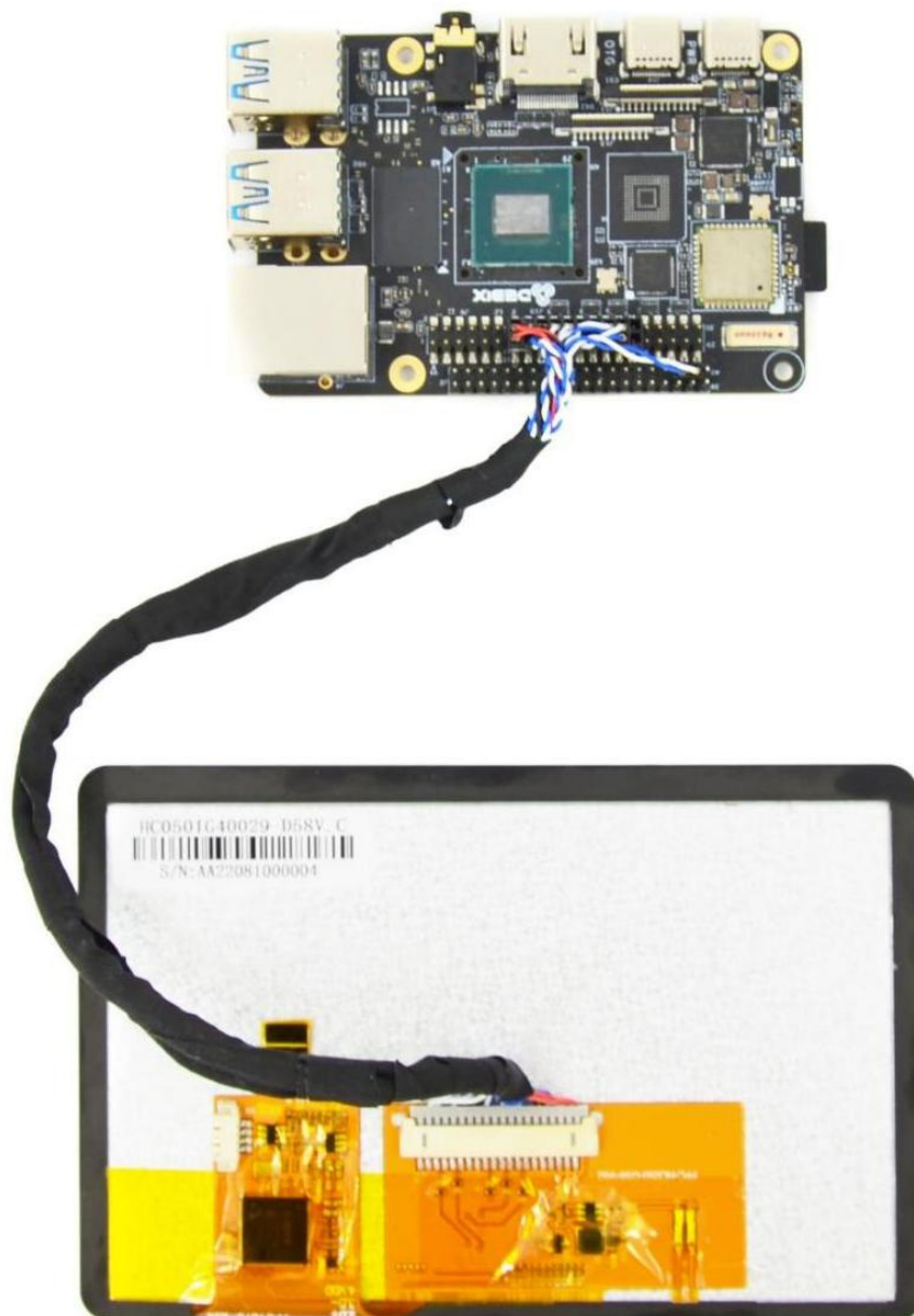
Figure 66 Connect LVDS screen cable to LVDS screen
