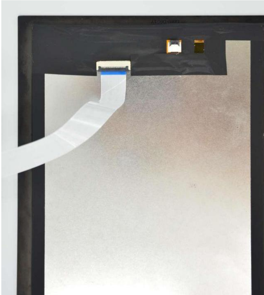
Figure 60 Connect FPC cable to MIPI screen
