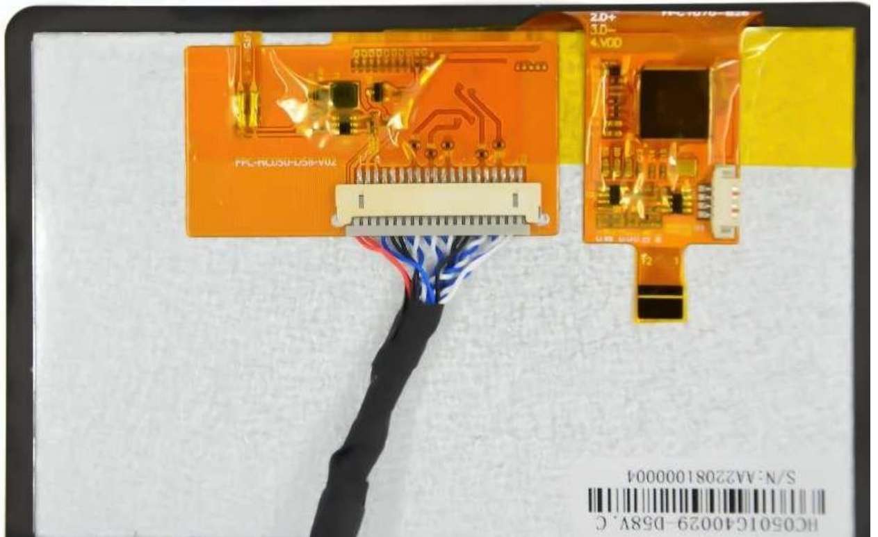
Figure 66 Connect LVDS screen cable to LVDS screen
