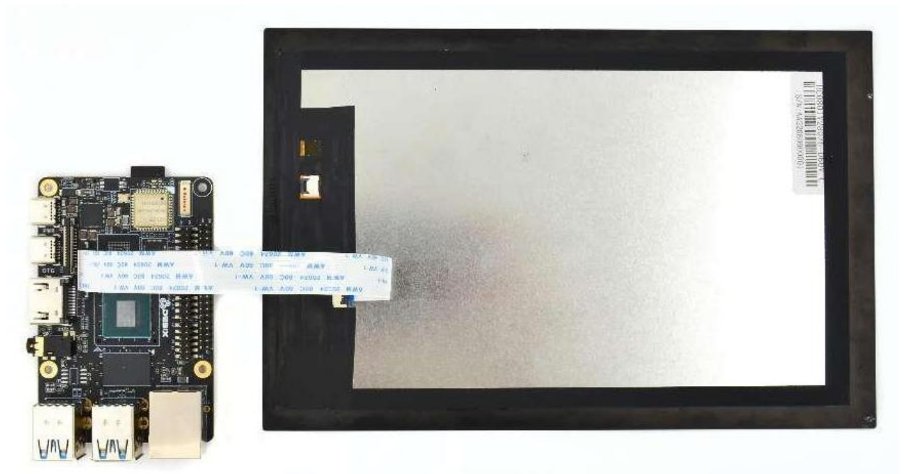
Figure 62 MIPI screen to DEBIX completed
