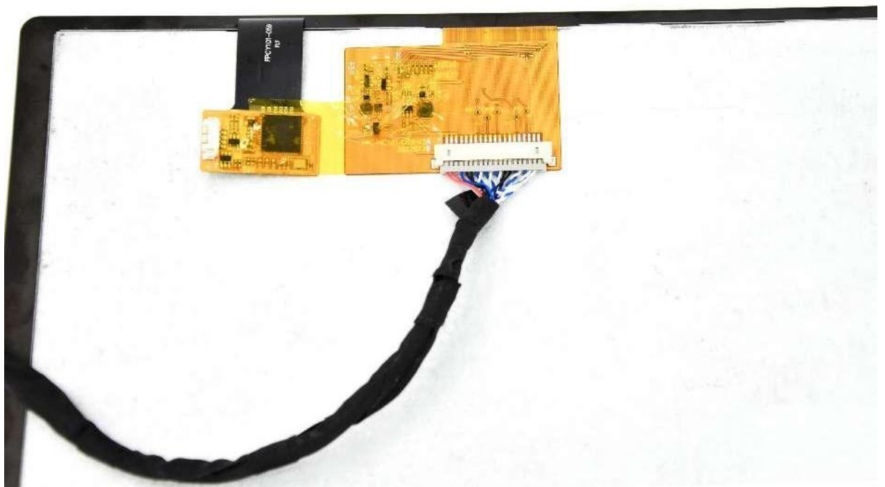
Figure 70 Connect LVDS screen cable to DEBIX
