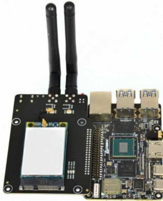
Figure 12 Connect DEBIX with DEBIX LoRa board
