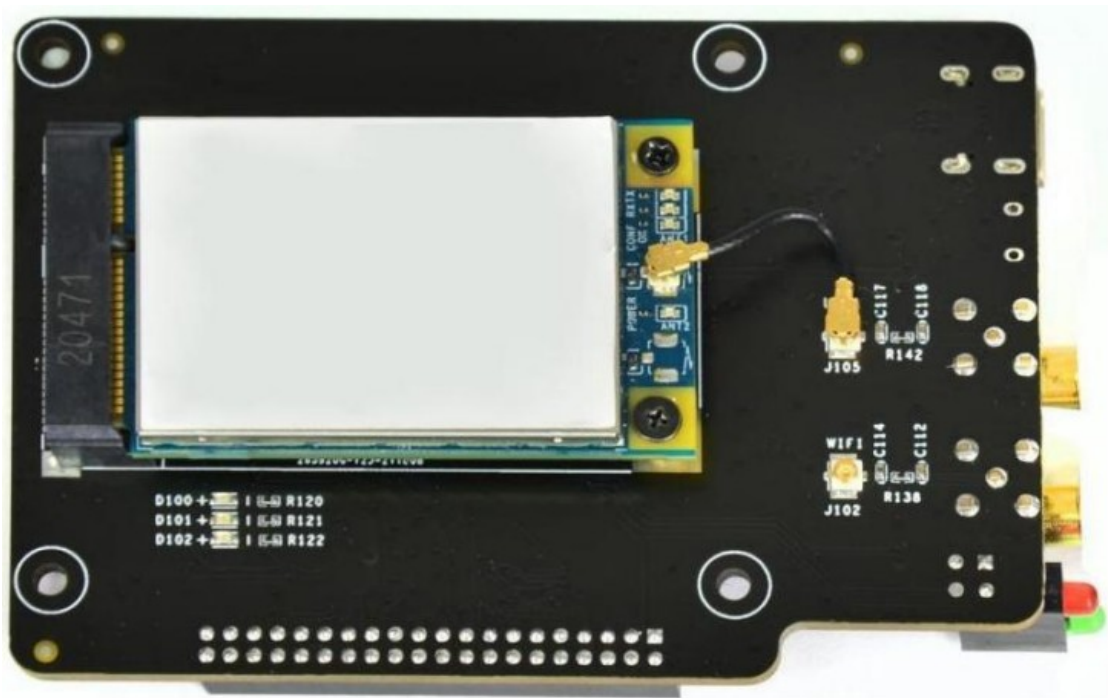
Figure 6 Connect DEBIX LoRa board with LoRa module
