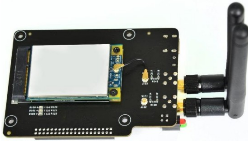
Figure 9 Connect DEBIX LoRa with antenna
