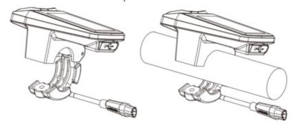
2. Adjust the installation angle for better visibility of the HMI screen while riding. Tighten the screw (M3\*12) to secure the HMI by M3 hex wrench. [Tightening torque: 1 N.m]
