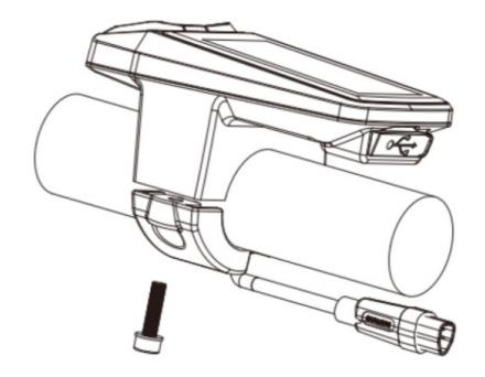
3. Connect the HMI with EB-BUS according to the symbols: F. HMI male connector; f. EB-BUS female connector.
