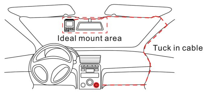
4. Use the installation tool to lift the edges of the windshield/molding and tuck in the power cable. Connect the Dash Cam to the car charger (plugged into cigarette lighter socket) and power cable.
