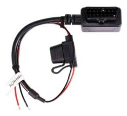
**Hardwired installation:** using the AHRHW Accessory cable, confirm the connections-12 Volts+ on the Red wire and chassis ground on the Black wireand confirm the 3 AMP fuse is good.
