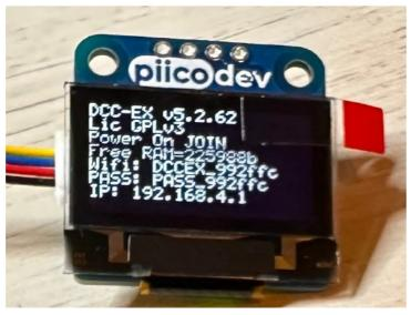
Please connect your smartphone or tablet to this WiFi network with the password shown on the OLED to begin running trains immediately! You have nothing further to do to start using your DCC-EX EX-CSB1. You can remove the protective cover on the OLED if you wish.
